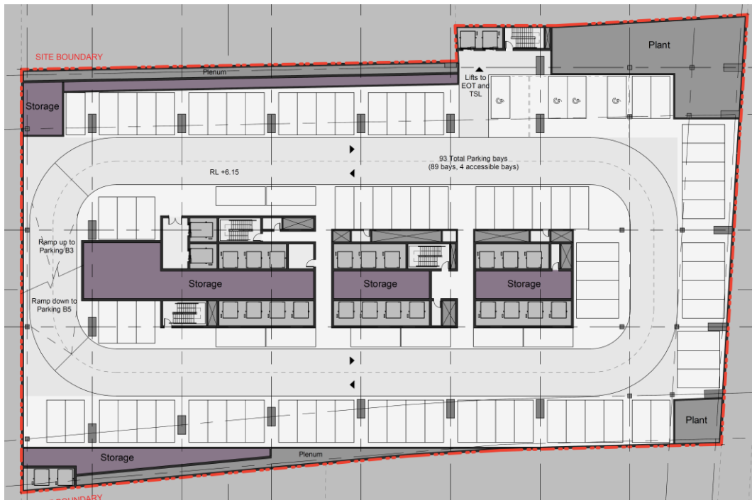
Figure 15: Parking layout – Basement 4 and 5
