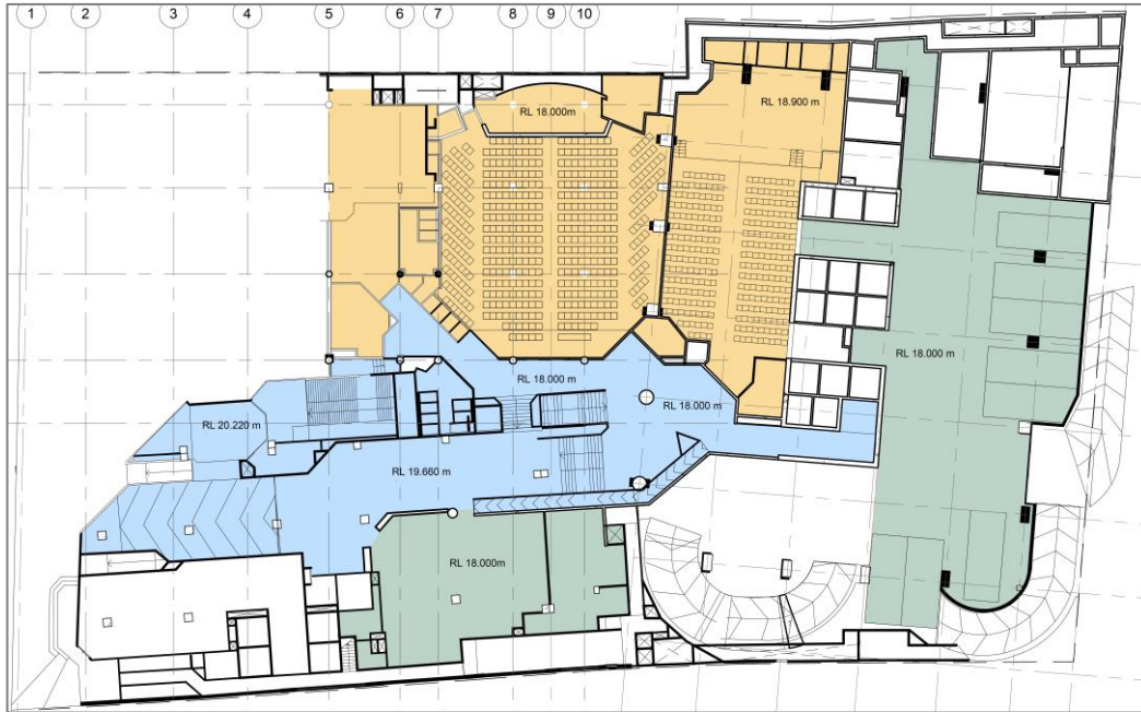
Figure 10: Existing parallel access ramps – Pitt Street level
